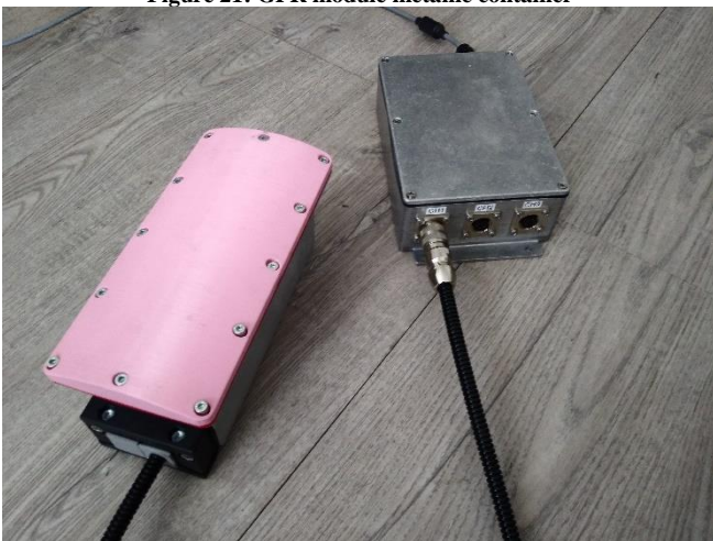
Figure 22: GPR module integrated in slot, covered with robust plastic plate (in pink), connected to IP65 sealed container for Radar Control Unit.
